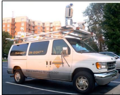
Figure 1: Mobile Imaging example: Transmap Mobile Mapping System
