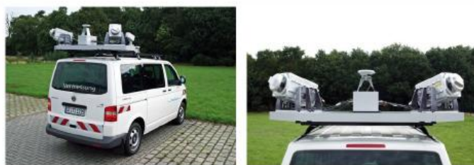
Figure 2: Optech Lynx operated by TopScan GmbH ( www.topscan.de )
